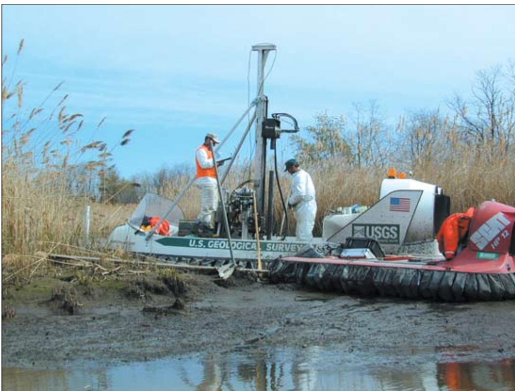
The USGS Hoverprobe is used to collect sediment cores to study long-term ecosystem history. Photograph by Daniel J. Phelan, U.S. Geological Survey
