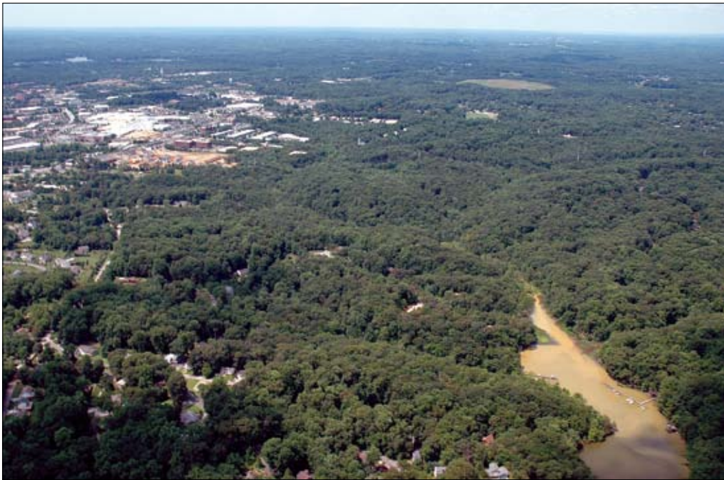
Plume of sediment-laden runoff, possibly from an adjacent construction area, near Annapolis, Maryland. Photograph by Jane Thomas, IAN Image Library ( www.ian.umces.edu/imagelibrary/ ).
